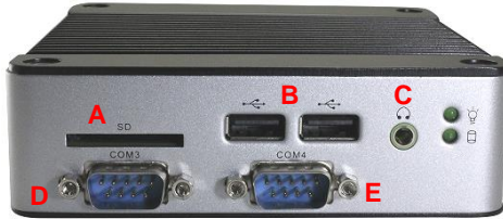
A: SD Card Slot B: USB 2.0 C: Line out D: COM or GPIO port E: COM, GPIO or CANbus port
