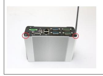
Step 3: Tighten the two screws on the back panel.
