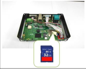
Insert the SD Card into the SD card slot.
