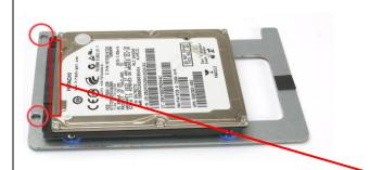
Step 5: Place the 2.5" SATA HDD on the Shockproof rings of the HDD
