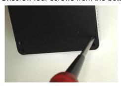
3. Unscrew two screws next to the VGA port at rear side.
