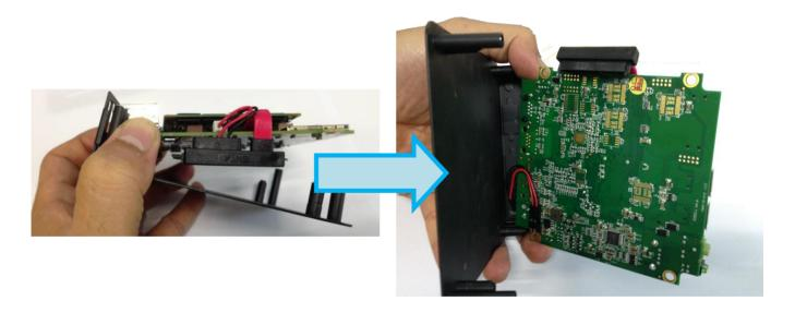
8. Connecting the SATA Cable to the cable connector and HDD power cable on the mainboard.
