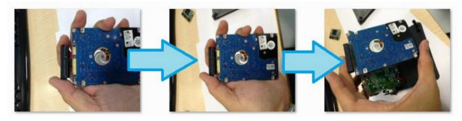
9. Bending the SATA cable and put the 2.5" SATA HDD under the main board.
