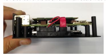
10. Use four small black screws from EBOX package bag to secure the 2.5" SATA HDD.
